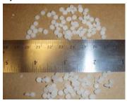
This product has a higher melting point (90 °C) which makes it ideal for seepage loss reduction in OBM wells over winter drilling programs and deeper applications (BHT below 90 °C). Seal-AX HT can also be utilized in WBM to coalesce other grades of LCM together to effectively create a more stable pill. It will also provide increased lubricity in directional wells.
