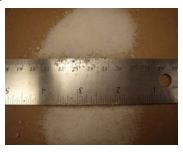
This product has a very high melting point (120 °C) and carries a charge. The product has primarily been utilized as an effective inhibitor in WBM, acting as secondary source of inhibition in conjunction with CES Envirobond (amine). In areas where hole stability is a concern, Polar-Whtie has been utilized to produce engineered filter cakes that significantly increase wellbore stability and provide wellbore strengthening.
