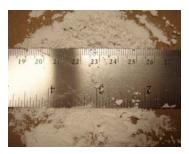
This product has a very high melting point (120 °C) and is micronized. The product has primarily been utilized to produce engineered filter cakes that significantly increase wellbore stability and provide wellbore strengthening.
