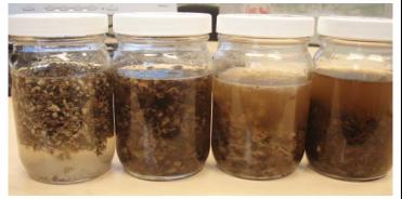
From left to right the jars contain cotton seed hulls with 30%, 20%, 15% and 0% Seal-AX<sup>™</sup> coating aged for a duration of three days in water. The discoloration is an indication of the degree of fiber breakdown and bacterial contamination. As displayed, even a 15% Seal-AX coating exhibits notably less decomposition as compared to untreated cotton seed hulls.
