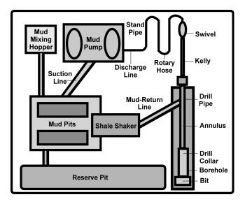
The drilling fluid system is the only component of the well facilities that remains in contact with the wellbore throughout the entire drilling operation. An effective drilling fluid system can minimize costs of drilling by reducing the number of days required on a wellbore. Using fluid that ensures wellbore stability while drilling can reduce the risk of excessive costs while drilling.
