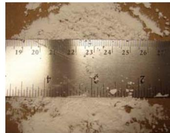
This product has a very high melting point (120 °C) and is micronized. The product has primarily been utilized to produce engineered filter cakes that significantly increase wellbore stability and provide wellbore strengthening.
