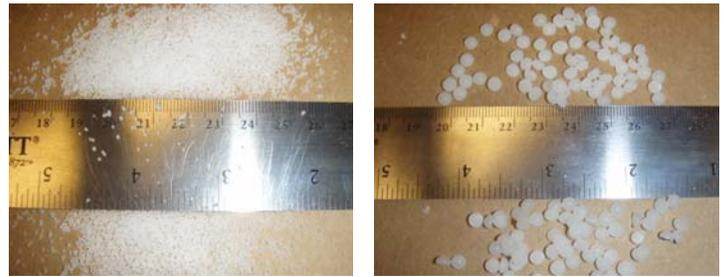
This product has a higher melting point (90 °C) which makes it ideal for seepage loss reduction in OBM wells over winter drilling programs and deeper applications (BHT below 90 °C). Seal-AX HT can also be utilized in WBM to coalesce other grades of LCM together to effectively create a more stable pill. It will also provide increased lubricity in directional wells.
