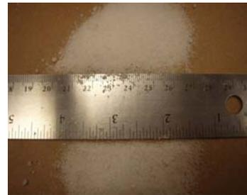
This product has a very high melting point (120 °C) and carries a charge. The product has primarily been utilized as an effective inhibitor in WBM, acting as secondary source of inhibition in conjunction with CES Envirobond (amine). In areas where hole stability is a concern, PolarWhite has been utilized to produce engineered filter cakes that significantly increase wellbore stability and provide wellbore strengthening.
