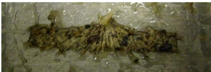
The pictures above are taken from the PPT. The CottonSeal™ slot illustrates a very tight, uniform compaction as compared to the cotton seed hull slot.
