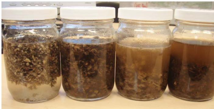
From left to right the jars contain cotton seed hulls with 30%, 20%, 15% and 0% Seal-AX™ coating aged for a duration of three days in water. The discoloration is an indication of the degree of fiber breakdown and bacterial contamination. As displayed, even a 15% Seal-AX coating exhibits notably less decomposition as compared to untreated cotton seed hulls.
